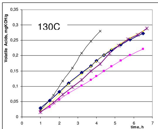
Fig 3: Oxidation Life test of oil from four GSU Transformers after 17-20 years of service Acidity <math>< 0.01 \text{ mgKOH/g}</math>, IFT $\approx 38 \text{ mN/m}</math>$
