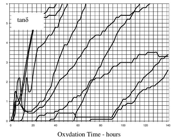
Fig. 2: Doble Free Life Test Behavior of different non-inhibited oils under operating temperature  $95\text{ }^{\circ}\text{C}$ . Rise of  $\tan\delta$  characterized the rate of producing conductive and polar by-products<sup>5</sup>
