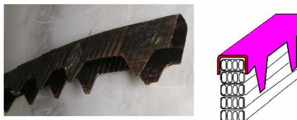
Fig 4: Hot spot area of winding of shell form transformer. Max. temperature at 50 °C ambient and 60 °C of top oil above 130 °C. All area contaminated with oil sludge
