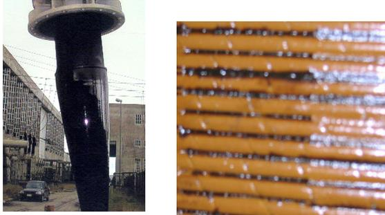
Fig 1: Sludge deposit of bushing porcelain (left) and winding (right)
